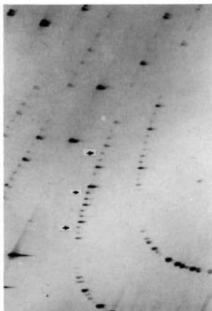
Fig. 3. A Weissenberg photograph of the ordered 12R structure (obverse and reverse) coalesced with 4H . Plate-like, intense spots are the reflexions of 12R (obverse), those marked with arrows are the reflexions of 4H and the remaining ones are the reflexions of 12R (reverse).
